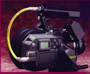
Aaton A-Minima camera showing the Oppenheimer "Swan Neck" and Battery Handle. The Power Cable is entering the camera through the rear L6. The accessory L6 is visible on the "Swan Neck".
